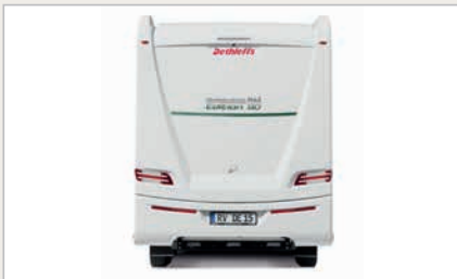
» Easy to repair: two-piece GRP rear
