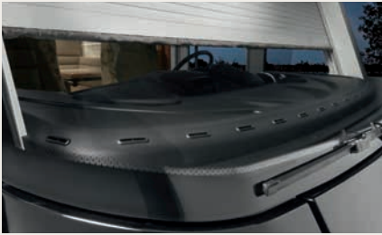
» Electric windscreen roller shutter and window defrosting
